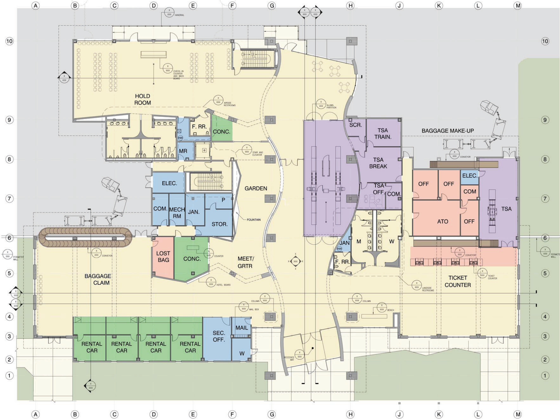
FIRST FLOOR PLAN SCALE 1/8"=1'-0" 0' 4' 8' 16' 32'
